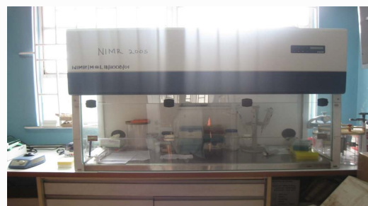
Type I biosafety cabinet containing PCR tubes and tips, micropipettes, micropipette stand and racks. Beside the biosafety cabinet to the left is a Stuart vortex mixer and a mini microcentrifuge.
